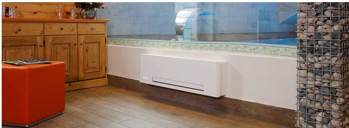
*Very often the traditional fanconvolution solution is not well understood by architects and designers because these systems occupy space for furniture and furnishings. With **ELIA WALL** we have the solution that allows you to have water system terminals installed at the top of the wall for summer and/or winter air conditioning without occupying floor space.*
